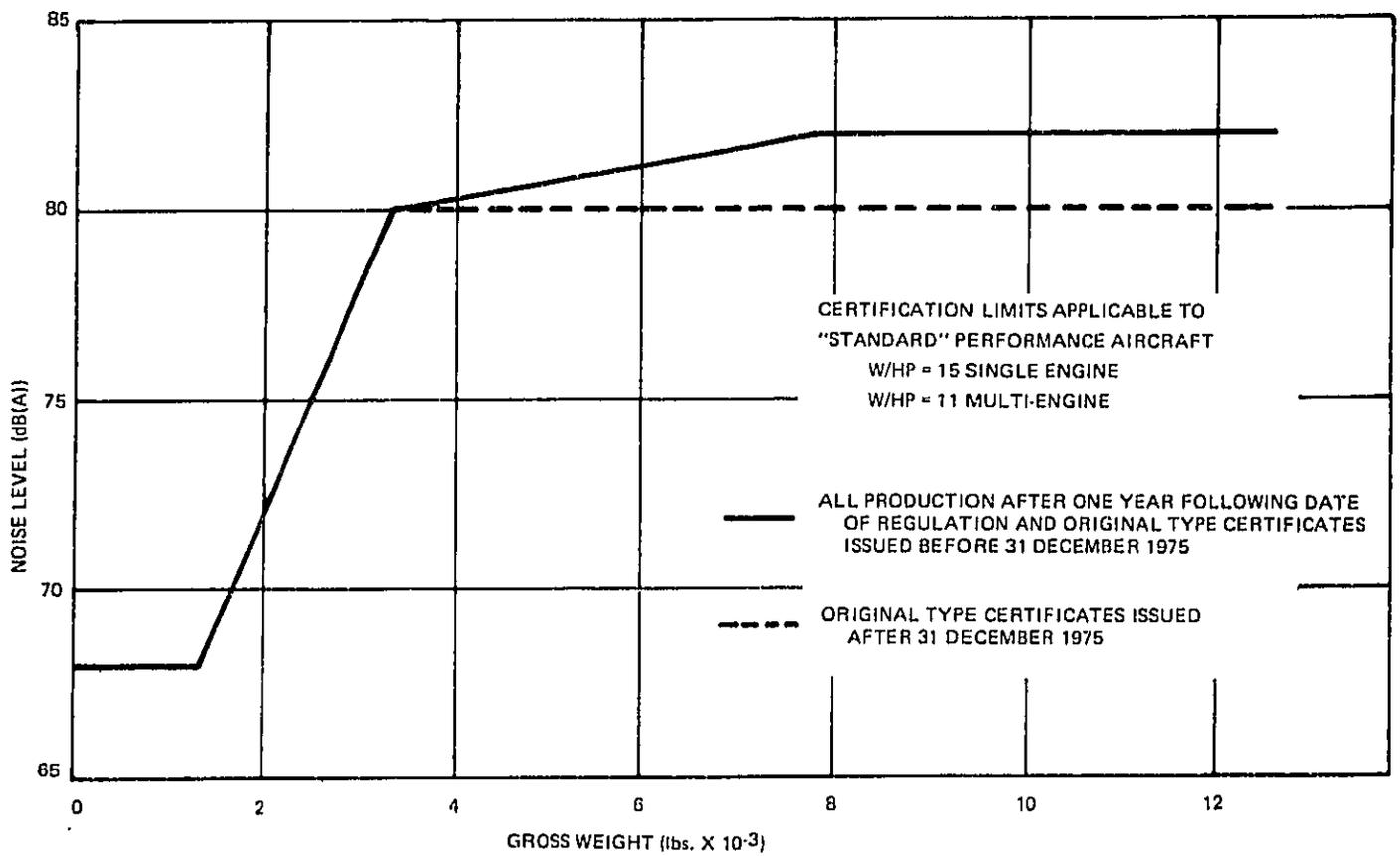
Figure 3-1. Proposed Noise Limits for Propeller Driven Aircraft
