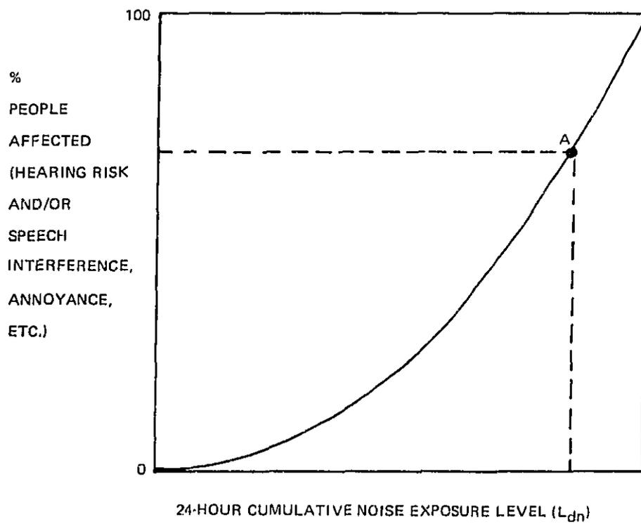
Figure 2-3. Generalized Curve for Determining Limiting Cumulative Noise Level For the Protection of Public Health and Welfare
