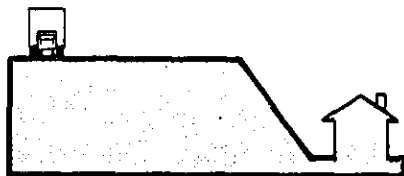
Figure 5.1-4. Shielding by an Elevated Highway or Railway.
