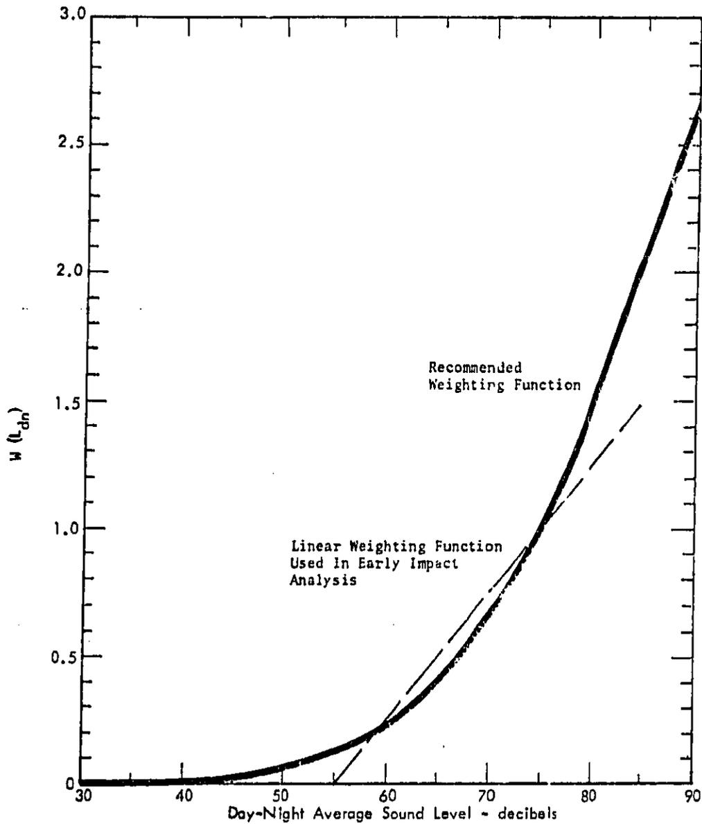
FIGURE VII-1. SOUND LEVEL WEIGHTING FUNCTION FOR OVERALL IMPACT ANALYSIS
