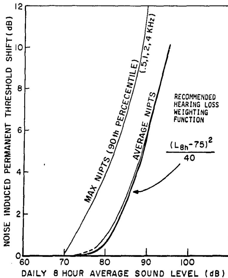
Figure VI-2. Potential hearing damage risk for daily exposure to 8 hour average sound levels. The curves predicts noise induced permanent threshold shift (NIPTS) in octave bands (.5, 1, 2, 4 kHz) for 8-hour exposure at various continuous noise levels. The eight hour average sound level can be replaced by DNL with negligible error if a person spends the remaining 16 hours out of 24 in  $L_{eq}$  of 70 dB or lower.
