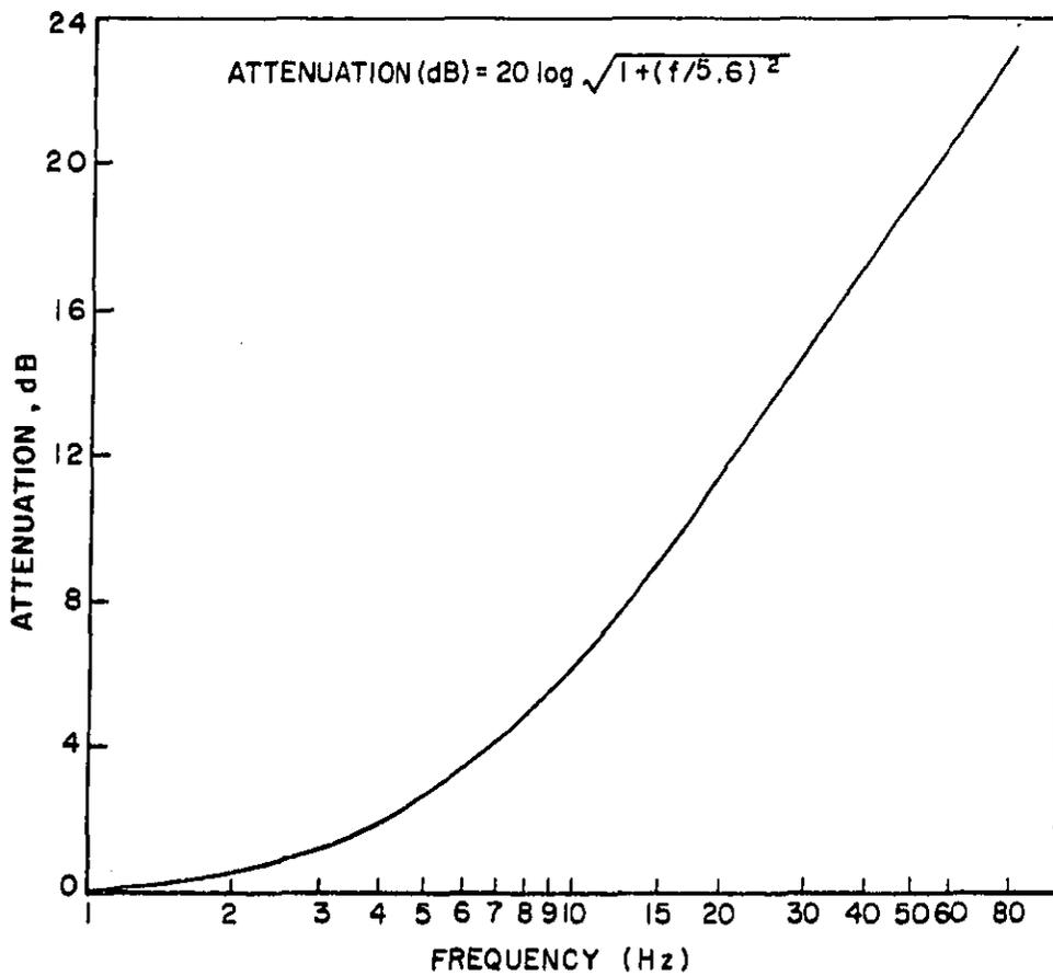
Figure V-1. Weighting characteristic for building vibration in terms of human response for the frequency range 1 to 80 Hz.
